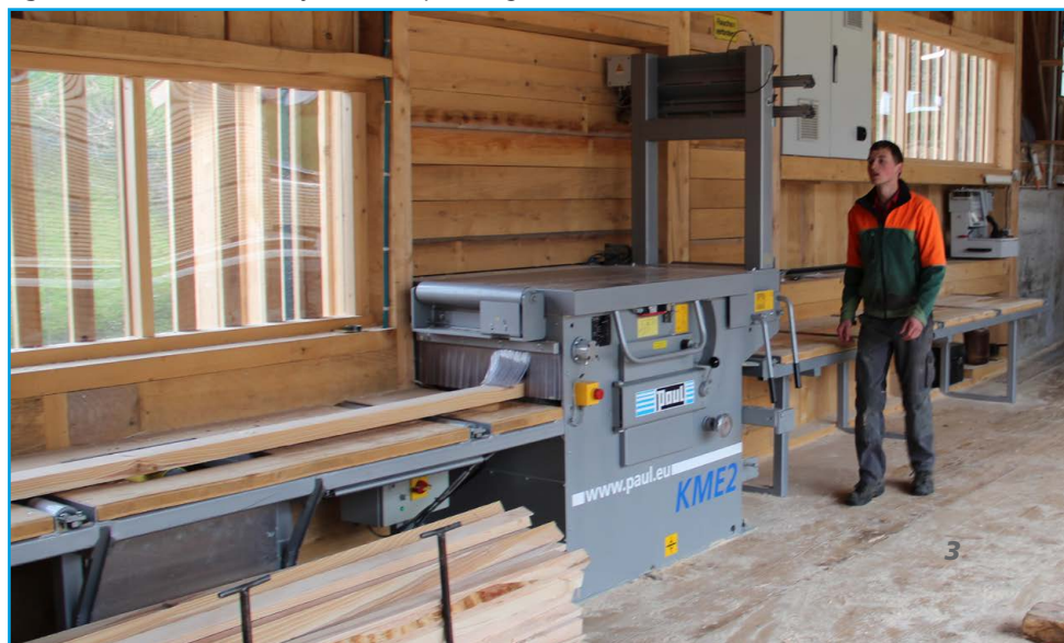
Fig. 2: KME2-750, manually loaded, operating in a sawmill
