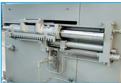
Fig. 20: Hydraulic saw positioning device
