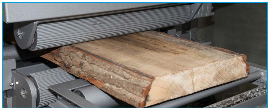
Fig. 16: Pinch roller unit
