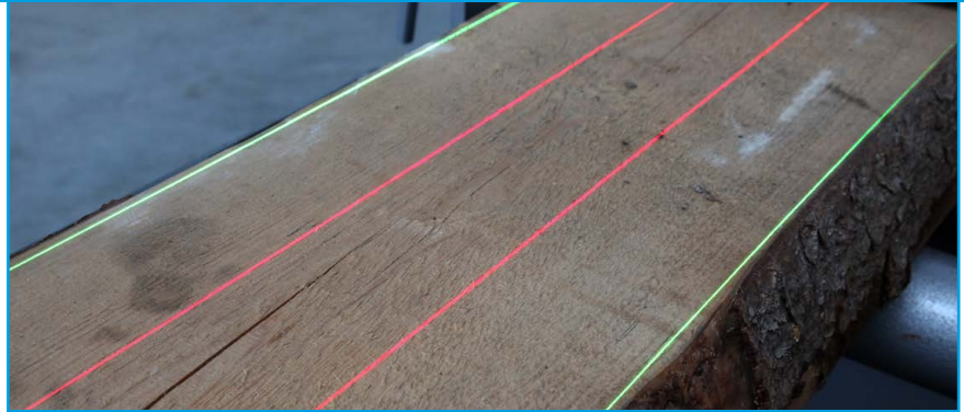
Fig. 15: Line lasers for ease of workpiece alignment
