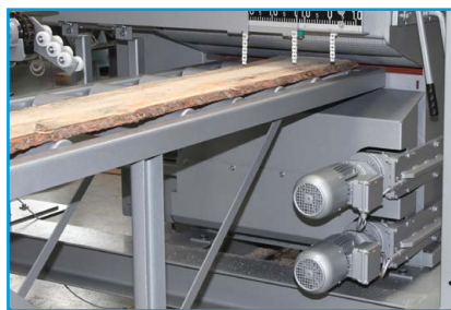
Fig. 21: Electric saw positioning device
