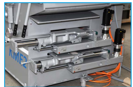
Fig. 22: Servomotor driven saw positioning device
